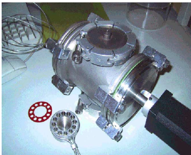
Fig. 2. The TAP sample holder with the chamber that contains the multiport valve.
